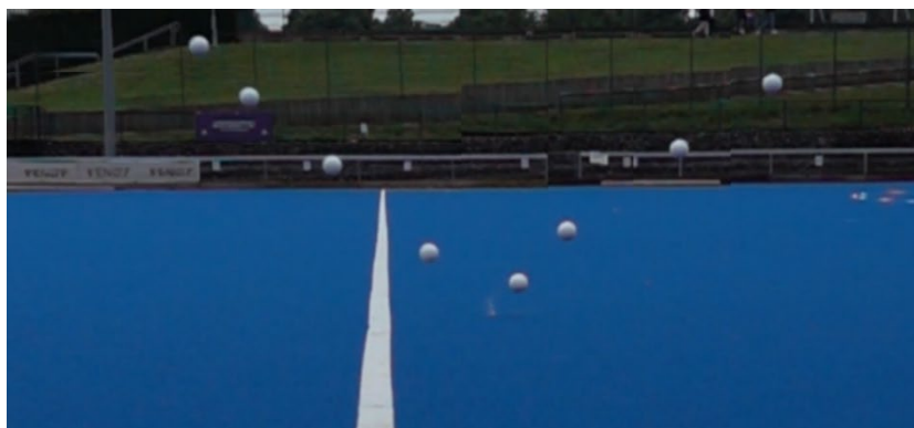
Figure 5. A composite image of the high-speed video footage of an oblique ball bounce
