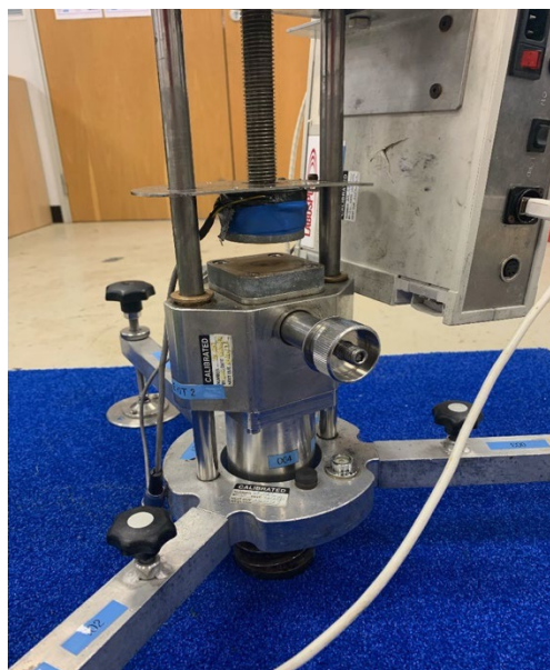
Figure 17. The modified AAA with a reduced drop mass of 10 kg and a reduced drop height of 20 mm
